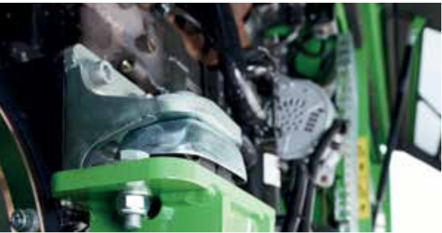
Low-vibration engine mounting reduces wear on components and lowers sound levels.
