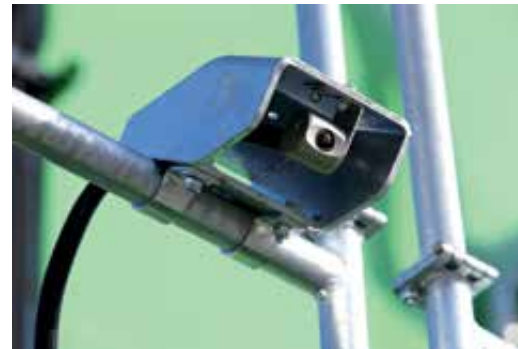
Dual cameras with views to the rear and to the right side are standard equipment.
